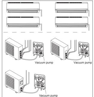
30, 36, 42Kunits use adapters that need to be installed at the indoor and the outdoor unit
